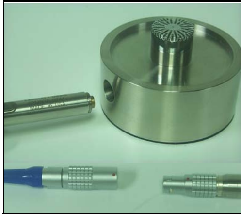
FIGURE 5-8 Preamp connecting to AEC100 and Extension Cable
