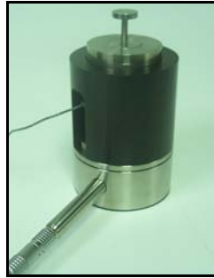
FIGURE 5-33 Artificial ear with vibrator and mass installed
