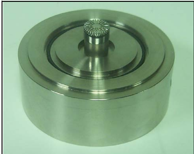
FIGURE 5-17 Microphone installed on AEC201
