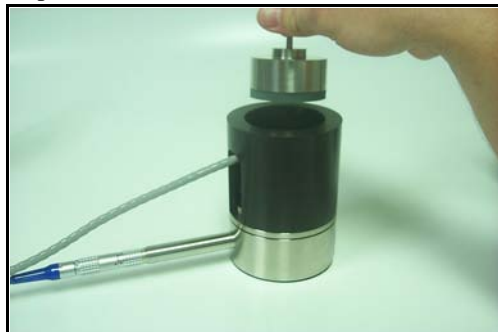
FIGURE 5-24 Mass being lowered onto headphone
