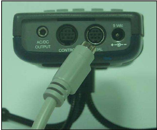
FIGURE 5-2 Connecting CBL006 to 824
