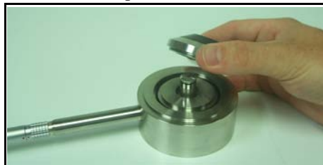
FIGURE 5-25 Coupler being installed on AEC201
