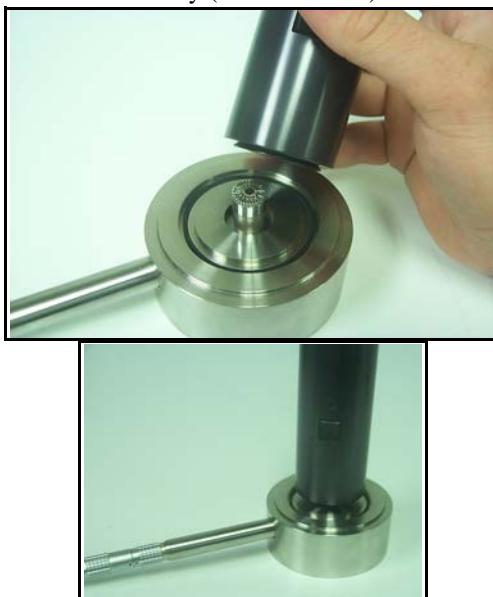
FIGURE 5-19 Installing the CAL250 on AEC201
