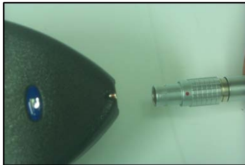
FIGURE 5-3 EXA010 extension cable approaching System 824
