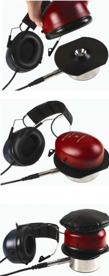
FIGURE 5-28 Sennheiser earphone and weight bag being installed on AEC201
