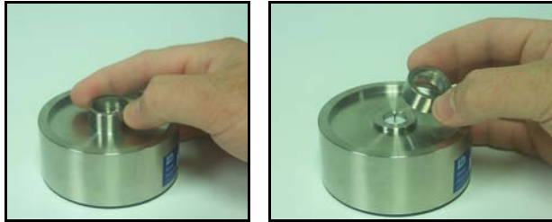
FIGURE 5-6 Protective ring being removed from AEC100
