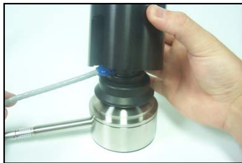
FIGURE 5-14 Retainer Ring being installed over headphone.
