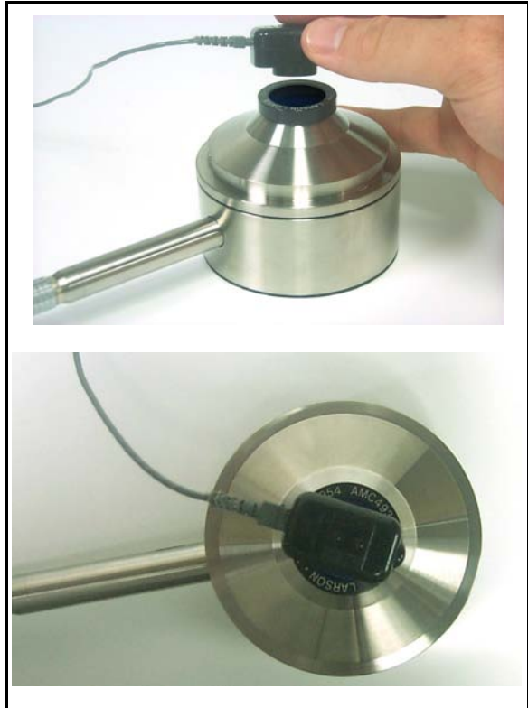
FIGURE 5-30 Vibrator being placed and centered on mastoid
