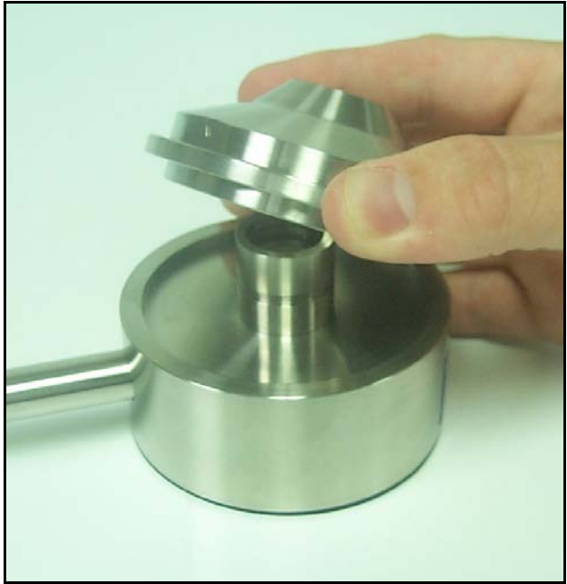
FIGURE 5-13 Coupler being installed on AEC100
