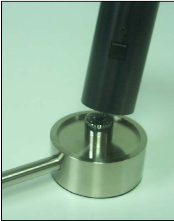
FIGURE 5-9 CAL250 being lowered onto 2575 microphone
