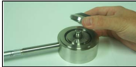
FIGURE 5-21 Coupler being installed on AEC201
