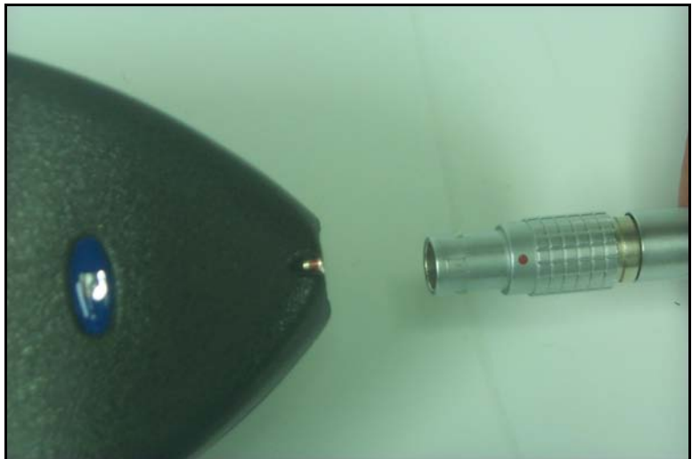
FIGURE 4-2 Connecting EXA010 extension cable to 824 and PRM902
