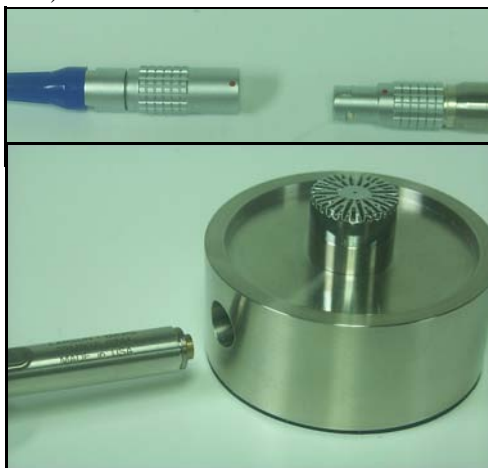
FIGURE 5-4 Preamp connecting to extension cable and to AEC100
