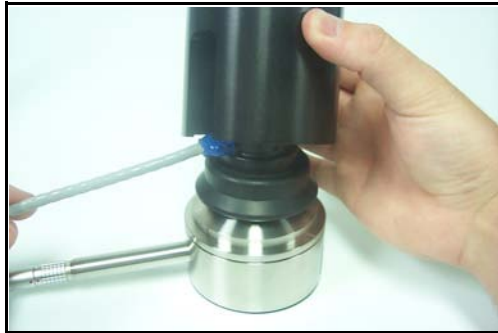
FIGURE 5-23 Retainer ring being installed on AEC201
