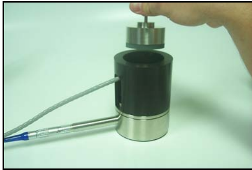
FIGURE 5-15 Mass being installed on AEC100.
