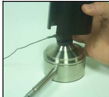
FIGURE 5-32 Retainer Ring being placed over vibrator
