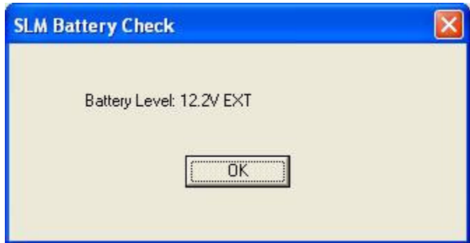
FIGURE 4-5 Battery Check Window
