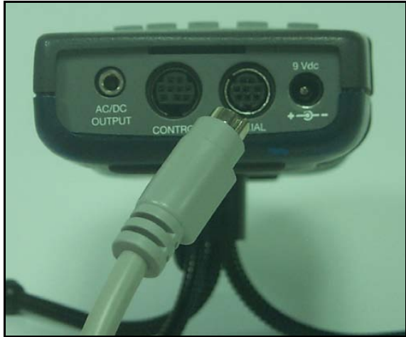
FIGURE 4-1 Connecting CBL006 to 824
