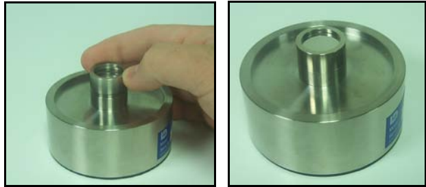
FIGURE 5-12 Installing Protective Ring on 2575 Microphone
